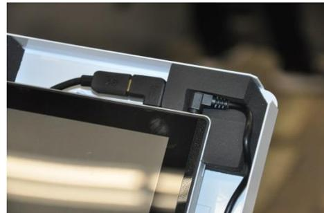
6. The tablet is placed in the tablet holder with the power on button on the bottom, left edge.
