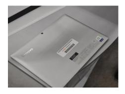
3. The tablet serial number is located on the transparent label.
